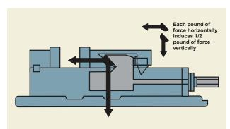
Down thrust "Semi Sphere Segment" mechanism eliminates jaw lift and work piece tilt. No need to hammer the workpiece as in other vices.
